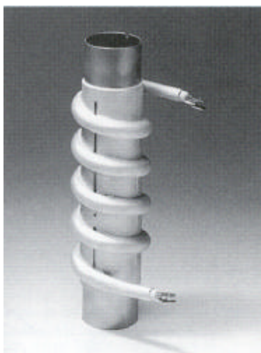
Figure 3: Paste-brazing of a continuous heater (aluminium to nickelised steel) in an inert gas
